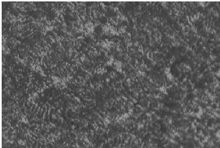
Fig. 9 A Magnetic Domain Image by Bitter Method
