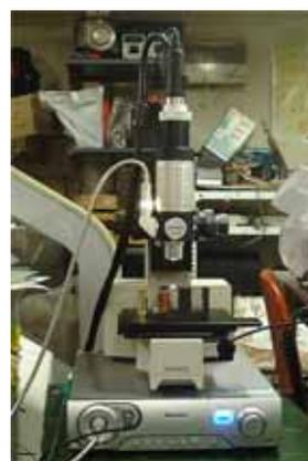
Fig.11 Experimental device for magnetic wall observation.
