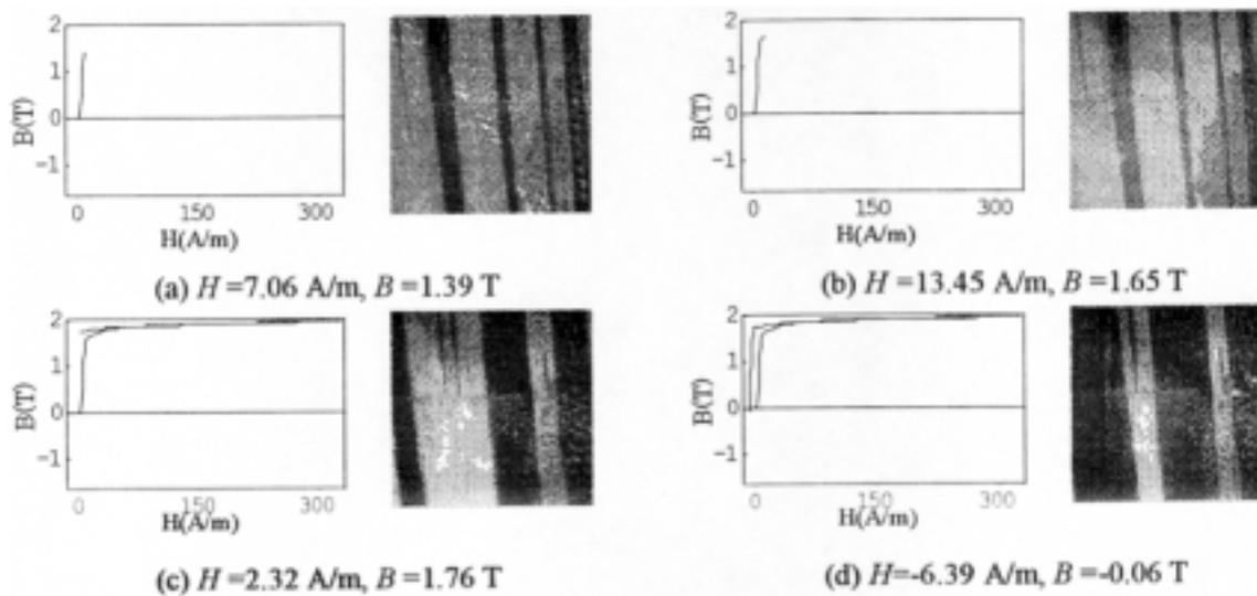
Fig. 6. Reconstructed domain images and magnetization curves.
