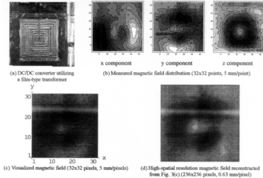
Fig. 3. Spatial resolution improvement of measured magnetic field distribution around a DC/DC converter.
