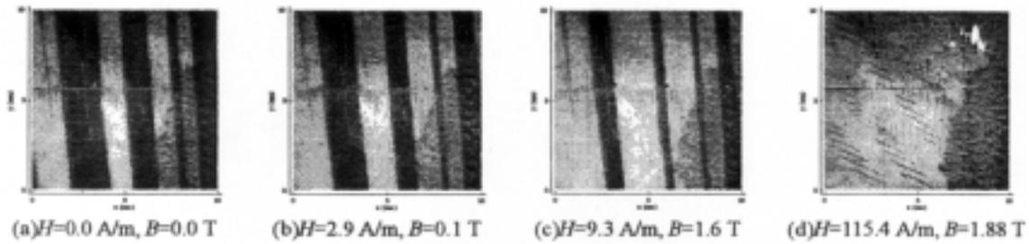
Fig. 4. Magnetic domain SEM images of the ORIENTCORE HI-B produced by Nippon Steel Co.(100 × 100 pixels, 0.1 mm/pixel).
