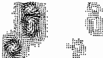
a) b) Figure 3 Current vector distributions: a) exact b) convoluted
