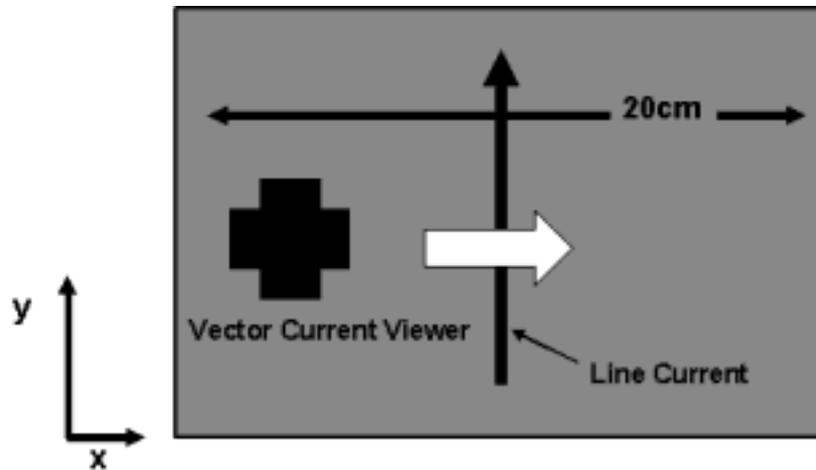
Fig.5 Experimental Verification for Spatial Resolution of Vector Current Viewer
