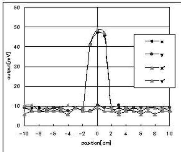
Fig.6 Spatial Characteristics (10kHz, 5A)
