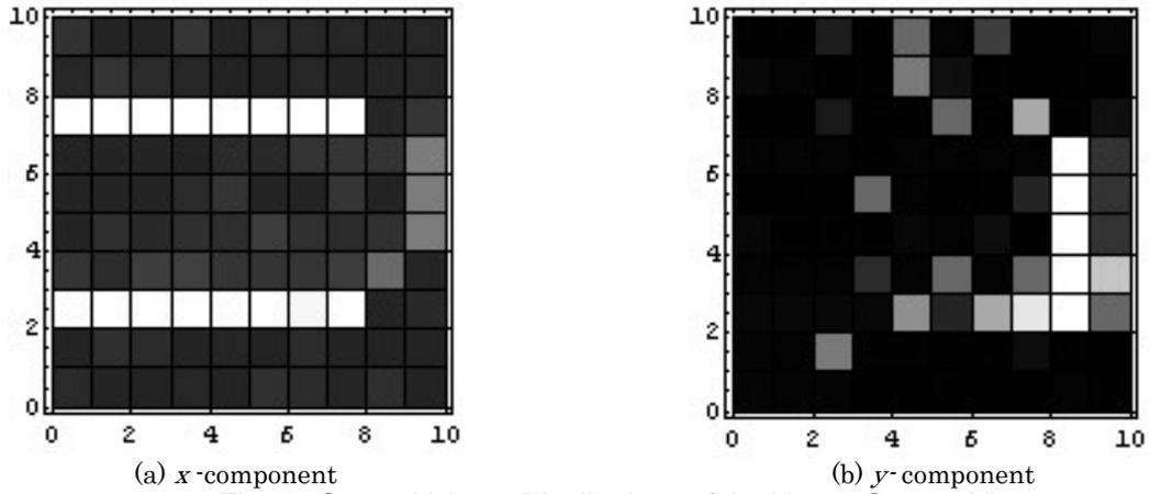
Fig.10 Output Voltage Distributions of the Vector Current Viewer (10kHz, 5A). White: High, Black: Low
