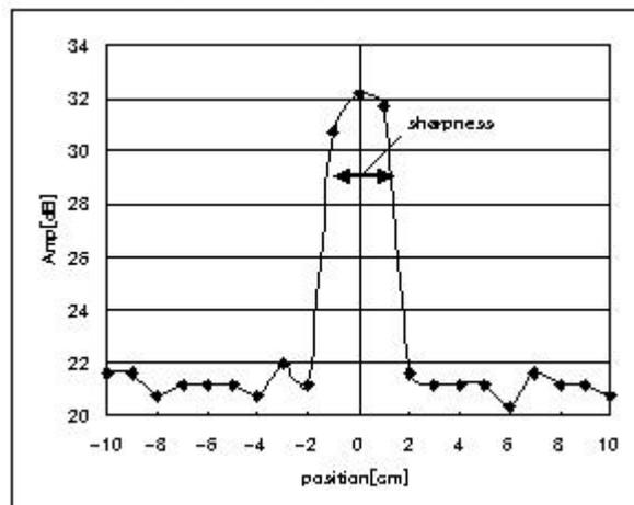
Fig.7 Definition of Figure of Sharpness
